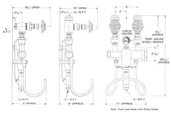
NOTE: A strainer and steam trap is recommended to be used in conjunction with all our steam mixing units. Foreign deposits in supply lines can effect ball check durability. Proper steam and water treatment is recommended to ensure proper performance and durability. Unit should be shut-off when not in use for extended periods of time.
