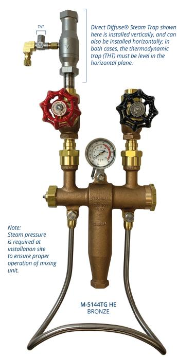
Maximum water temperature: 200°F (93°C) Maximum working pressure: 150PSI
