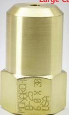
The B-25 Nozzles are of two piece construction with large tangential metering slots in the internal Disc to give a nonrestricted flow with a uniform "Solid" distribution. For special applications, a hollow cone spray can be produced from this same design. These Nozzles with high flow rates and coarser sprays are used in gas scrubbing, adsorption towers, brine spraying, and chemical and industrial processing.
